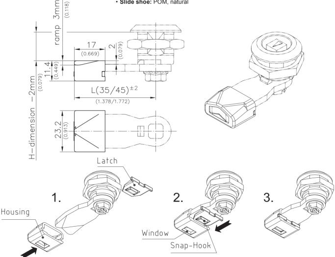
The Housing will be pushed onto the cam until it alines with the cam. The Latch will be pushed underneath the cam into the remaining space until the snap-hook is latched into the window audibly.
