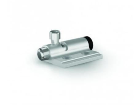
Bolt can be held back in unlocked position. Body: clear anodised aluminium. Shaft and handle: raw aluminium. Cap: PE, black. Spring: stainless steel.
